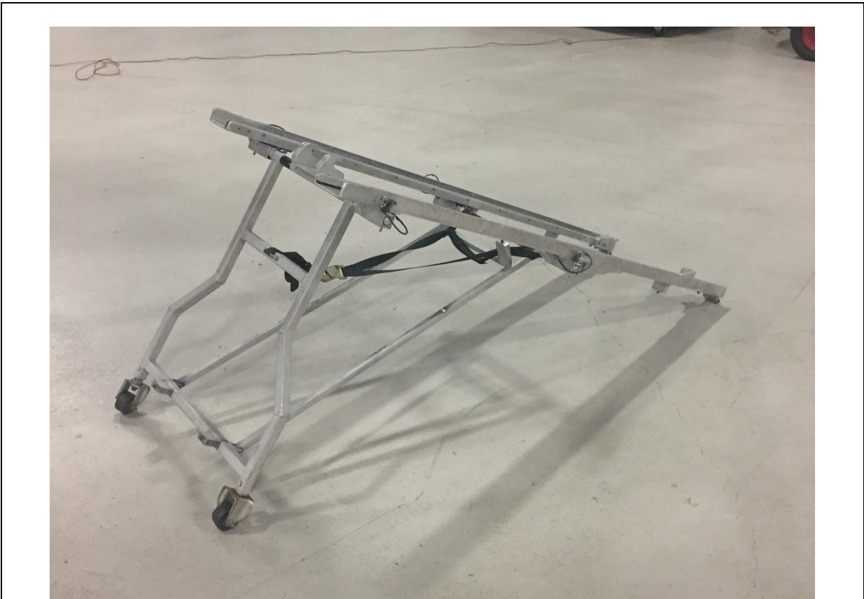
Figure 18 – Stretcher bridge used to load the Ferno drop-leg stretcher
